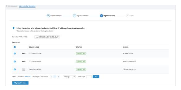
Step 4 Verify that all the migrated devices are visible and connected on the new controller. When all the migrated devices are in Connected status on the **Device** page on the new controller, click **Forget Devices** to finish the migration process.
